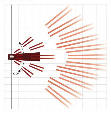
Volumetric detectors are specified if the monitoring activity primarily focuses on covering a large surface. The most suitable ADPRO PRO E-detector can be selected accordingly from the extensive product range based on the nominal detection distance, number of zones (fingers) and the monitoring angle.
