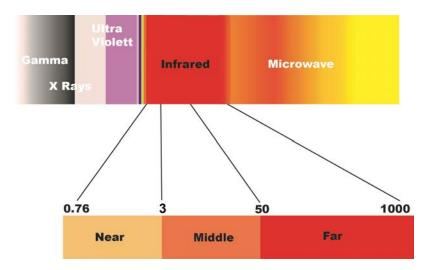
As the graph shows, infrared radiation can be broken down into three categories: near-infrared (IR-A: 0.78...1.4 μm / IR-B: 1.4...3.0 μm, mid-infrared (IR-C: 3...50 μm) and far-infrared (also IR-C: 50...1000 μm).
