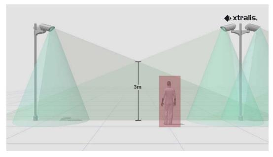
A main alarm is only triggered when two or more detectors generate an alarm signal. Use of this option requires precise analysis and project design. If implementation is not optimal, there is a risk that no alarms will be triggered, i.e. very thick fog between the two detectors.
