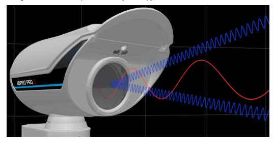
People and animals emit infrared radiation at a wavelength of approximately 10 micrometers (µm). The sensor circuitry and sequence of software algorithms in the detector are calibrated in a way that ensures recognition and analysis of these wavelengths only. They also detect the temperature differences in a defined detection area between the background and the moving object.
