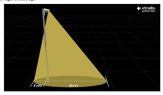
The detectors provide dedicated monitoring of the creep zone, particularly in corners and geometrically complicated applications. The creep zone is covered additionally by a second detector on the bottom face of the housing.
