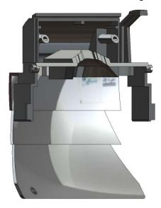
This zone can be shaped like a curtain or barrier for perimeter monitoring or as a broad fan for monitoring a large surface or volume. The optical system splits the IR radiation into several axes according to the desired geometry of the monitored zone (in comparison, a camera or a telescope has only one axis).
