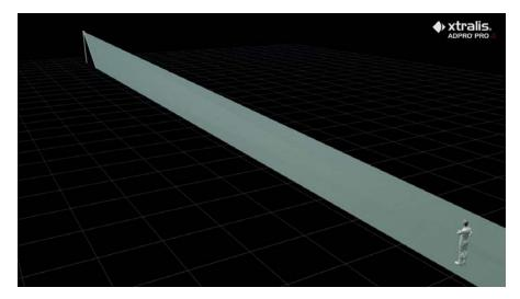
This type of monitoring is characterized by a detection zone that extends for a significant distance across a narrow width. Barrier detectors are specified when the main priority is to monitor clearly defined boundaries. As this type of detector is also capable of detection within its narrow monitoring zone that extends for a significant distance, it is also referred to as a volumetric detector. For clarity's sake however, it is referred to as a barrier detector in Xtralis documentation.
