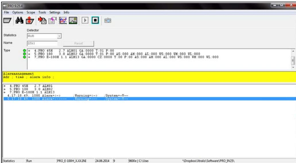
List of all connected detectors, their types, Firmware version and number of alarms since beginning of recording. This example shows three Detectors connected, 4 and 5 have one Temper (T: 01) Alarm in the counter ("T: 01") The events are listed real time below (4 and 5 "System=-V" for Vandal).
