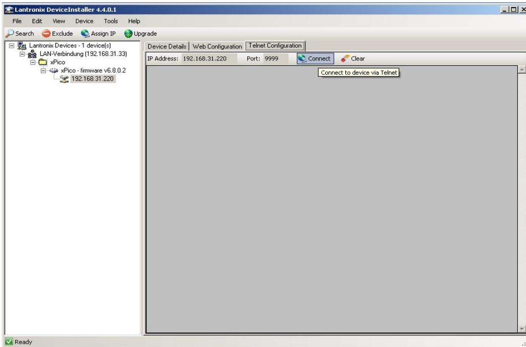
4. Press **Enter** within the first 5 seconds after connecting to enter the device setup mode as shown below, otherwise the telnet server on the xPico module will disconnect and should be connected again:
