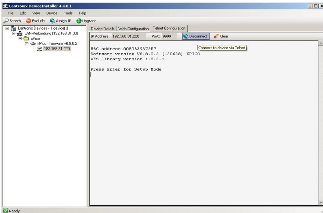
Upon successful connection to setup mode on the xPico module, an option menu appears.
