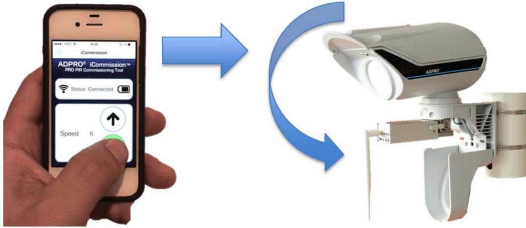
When the detector has full performance across the desired range, the vertical alignment is done and the iCommission unit can be removed. Continue with the commissioning process.
