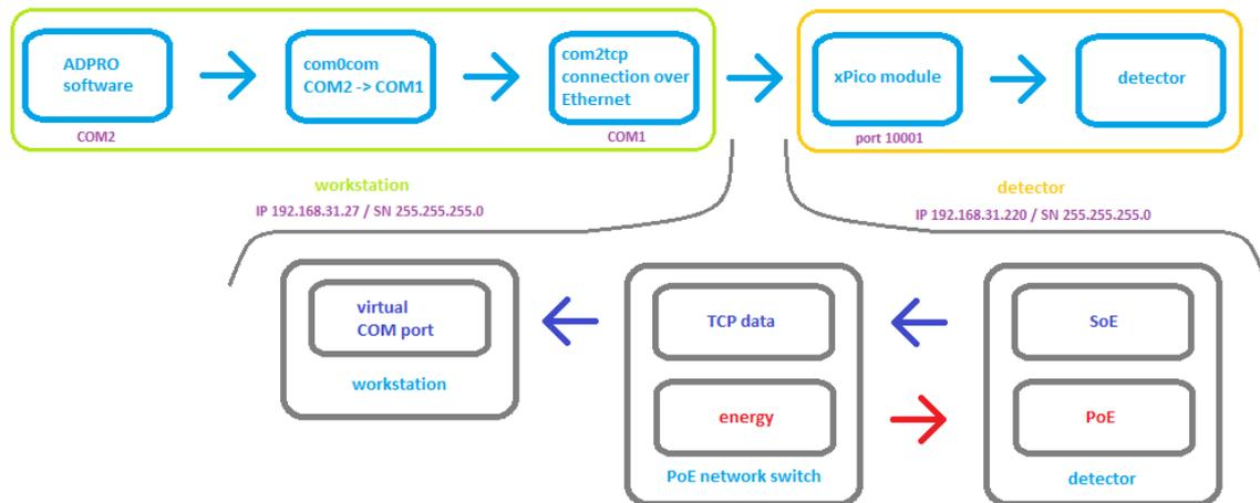
This overview shows all three parts of the system: the workstation, the PRO E detector and the data infrastructure in-between.
