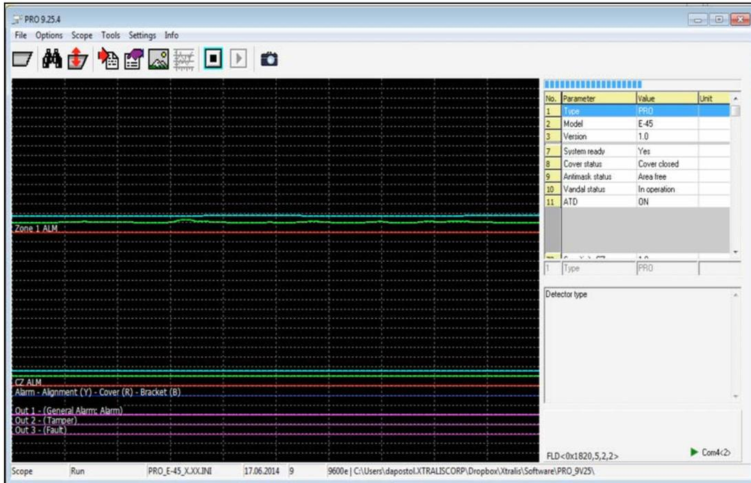
The Scope view illustrates the cause/response relationship between inputs and output. The view shows all signals and their levels on a time axis; it allows for a detailed analysis of the detector's operation.
