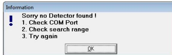
Make sure you’ve selected the correct COM port (in which case the TX LED of the bus interface module should be blinking during the search and the RX LED should be blinking if a detector is found) and that the search range covers the detectors’ addresses. Click “OK”, check for errors, and repeat the search.
