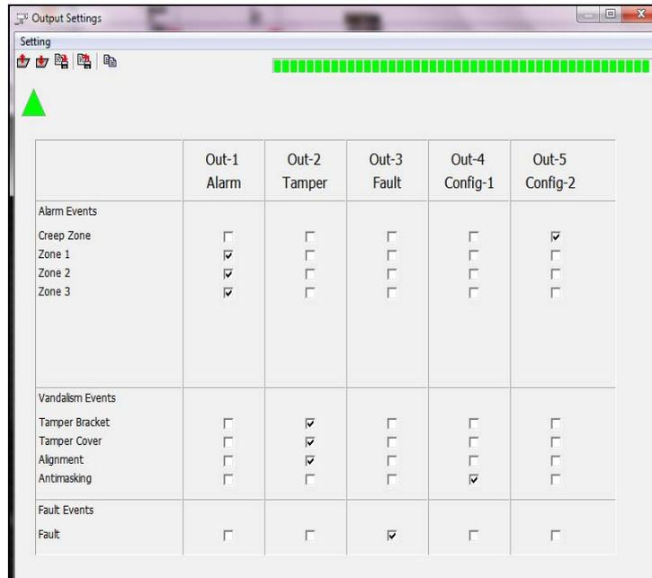
1. Alarm: Zones 1-3 (here: L, M, S) trigger output 1.
