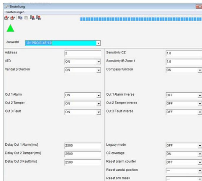
Content and layout are detector-model-dependent and primarily designed to review and change the detector’s parameters. These include address, sensitivity, output functions, etc.
