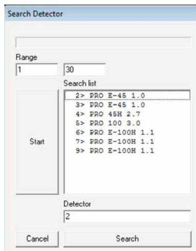
**Note:** Detectors are given IDs (addresses) in the range of 1 to 254. It is recommended to narrow down the range when searching for a detector so as not to take time and retrieve the connected detectors more quickly.
