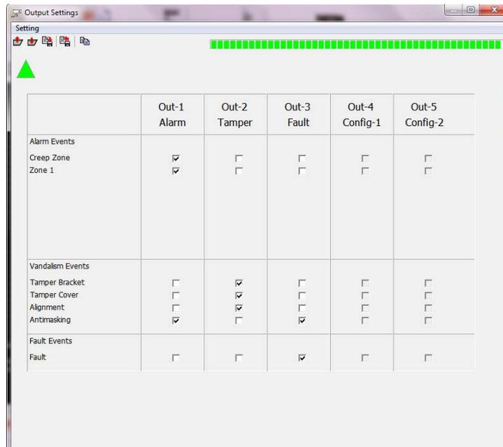
1. Alarm: 360PROtect™ (creep zone and behind detector) and main zone trigger output 1. Anti-masking triggers output 1 as well, but together with output 3.
