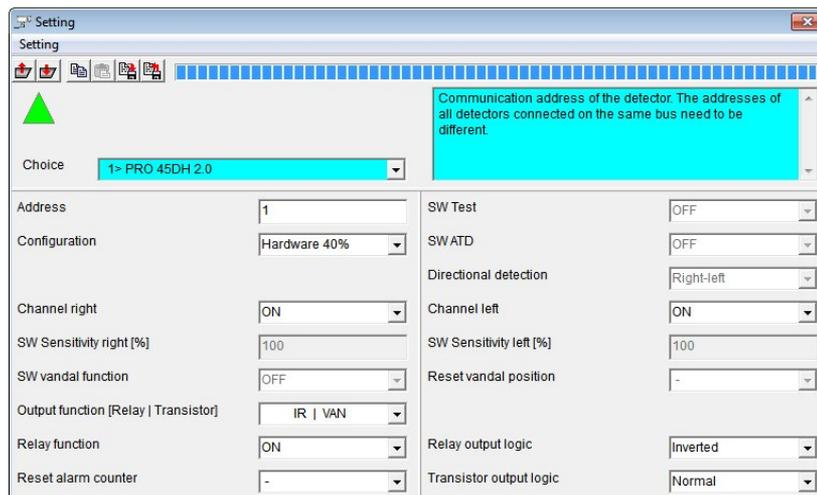
**Note:** Several of the PRO detector settings have the prefix “SW”. This indicates, that they can be set here in software, but also in hardware through DIP switches.
