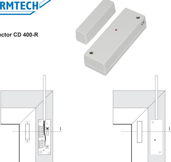
Magnet should be placed axially, opposite to connectors 6-10.
