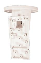
Surface-mount the swiveling B338 plastic ceiling mount to the ceiling. It is suitable for use with many detector types. The vertical swivel range is +7° to -16°, while the horizontal swivel range is ±45°.
