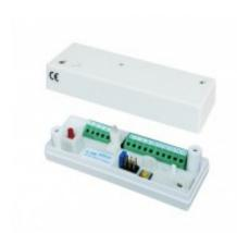
IU 400 is an interface/analyzer for glass break detector GD 475. It has three relays one for Intrusion, one for Fault and one for Tamper. Max 10 units of GD 475 detectors can be connected to one IU 400 unit. IU 400 together with GD 475 is certified according to EN 50131-1 and EN 50131-2-7-2:2013 Grade 3, Class II.
