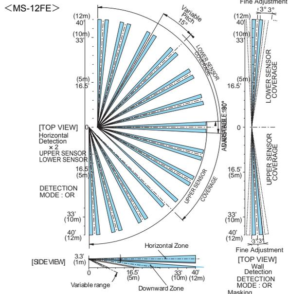
Detection distance is set by adjusting the angle of downward zone.
